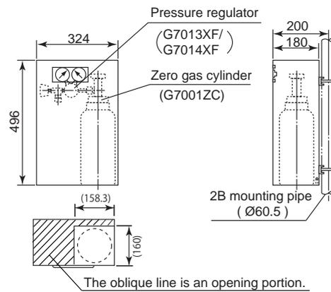
(Note) The zero gas cylinder and the regulator valve are not included in the E7044KF (case assembly)
