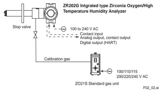
Note: The installation temperature limits range for integrated type analyzer is -20 to 55°C.
