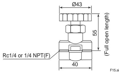
**15. K9292DN /K9292DS Check Valve for Calibration-gas line**
