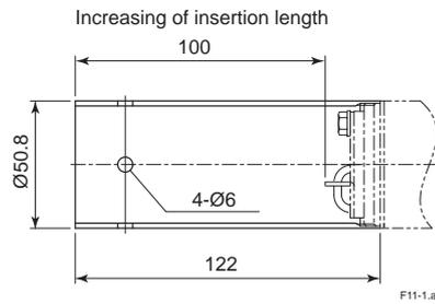
9. Model ZH21B Dust Protector for High Temperature Humidity Analyzers
