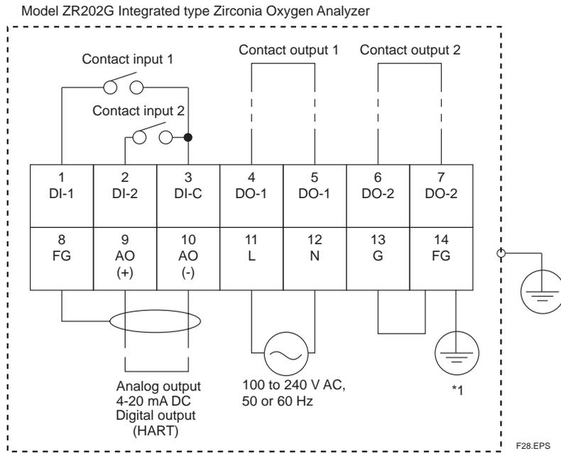
The protective grounding for the analyzer shall be connected either the protective ground terminal in the equipment or the ground terminal on the case.
