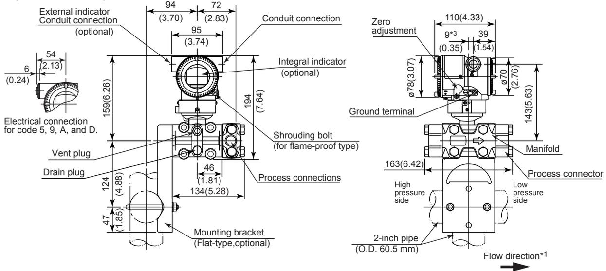
\*1: When Installation code 2, 3, or 8 is selected, the flow direction on above figure is reversed. (i.e. the arrow faces to the left [ ← ])
