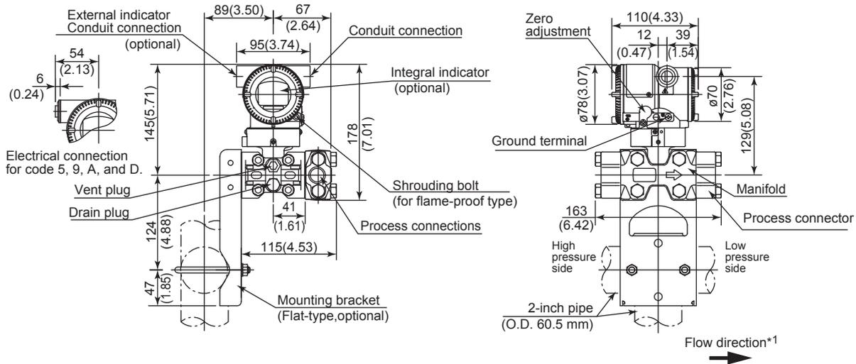
\*1: When Installation code 2, 3, or 8 is selected, the flow direction on above figure is reversed. (i.e. the arrow faces to the left [ ← ])
