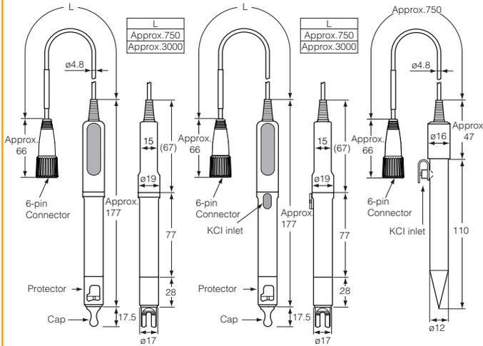
Test tube size pH sensor
