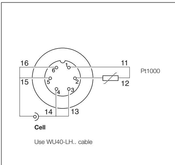
Figure 2. Wiring diagram threaded models
