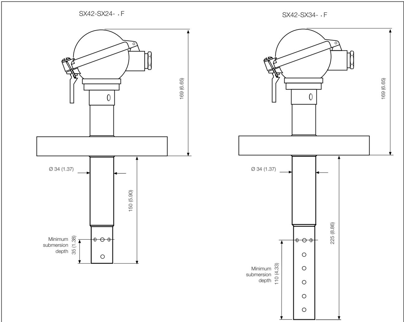
Figure 4. Flanged models (flange dimensions see fig.5)
