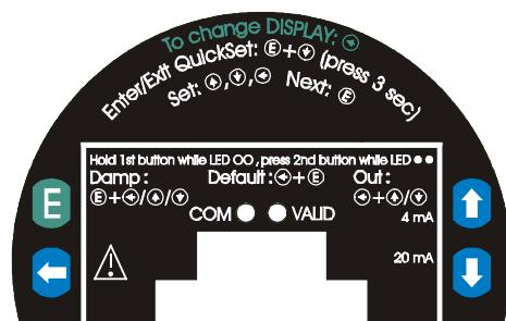
Procedure of programming: press button in the relevant sequence and check the state of the LED-s. Symbols for the states of the LED-s:
