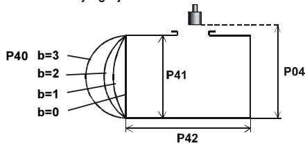
Standing cylindrical tank with conical bottom  $a = 1 ; b = 0$
