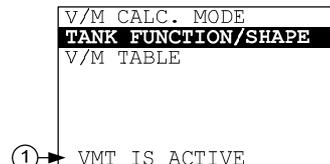
All modifications are done on a temporary table. This temporary table becomes valid after exiting. Modifications during the programming procedure have no effect on the measurement and the transmitting.
