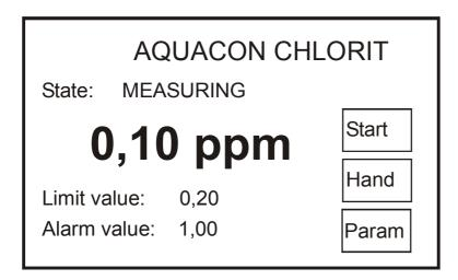
The automatic analysis cycle can be interrupted at any stage by touching the button "Hand" or the button "Param" on the touchscreen (see 3.5). After the finish of the analysis, the new measured value will be displayed on the touchscreen and the analyzer state is changed to "STANDBY".
