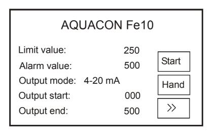
In parameter mode, a new screen will be displayed which shows the parameters Limit value, Alarm value, Output mode, Output start and Output end. By touching the button ">>", a second screen will be displayed with the parameters Sampling interval, Calibration factor, Rinse time and Reagent volume.
