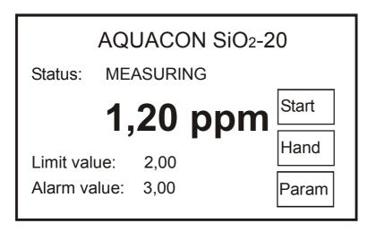
The automatic analysis cycle can be interrupted at any stage by touching the button "Hand" or the button "Param" on the touchscreen (see 3.5).
