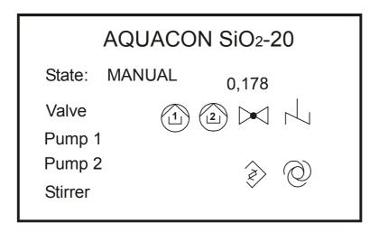
During manual operation, the pumps, the sample inlet valve and the stirrer can be activated/deactivated by touching the appropriate symbols. The active part will be displayed with inverse letters.
