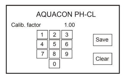
To leave the screen and confirm/safe the new parameter value, the button "Save" must be touched.
