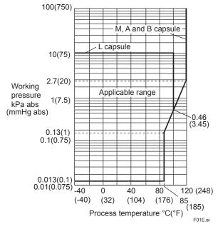
Figure 1. Working Pressure and Process Temperature
