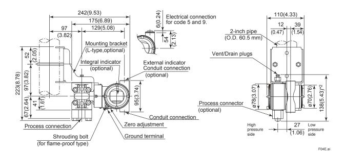
Horizontal Impulse Piping Type (INSTALLATION CODE '9') (For CODE '8', refer to the notes below.)
