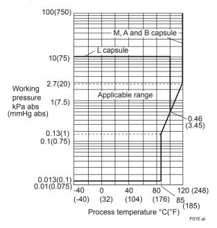
Figure 1. Working Pressure and Process Temperature
