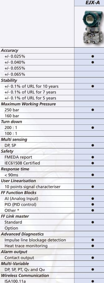
[\* Other FB include SC (Signal Characteriser), IT (Integrator), AR (Arithmetic) and IS (Input Selecor)]
