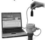
The IrDA adapter and the IrDA port of the device must be placed whithin a 5...50 cm distance and facing each other!
