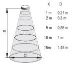
Diameters corresponding to 5° beam angle.
